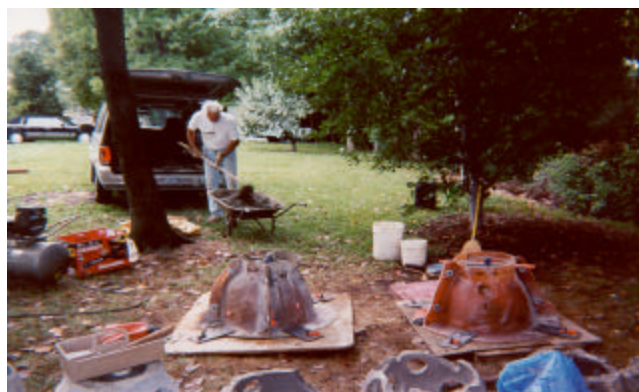
Reef Ball Mold System at Work in Bob's Backyard
