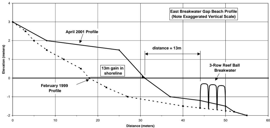
**Figure 4. Beach Profile across Breakwater near East Gap**
