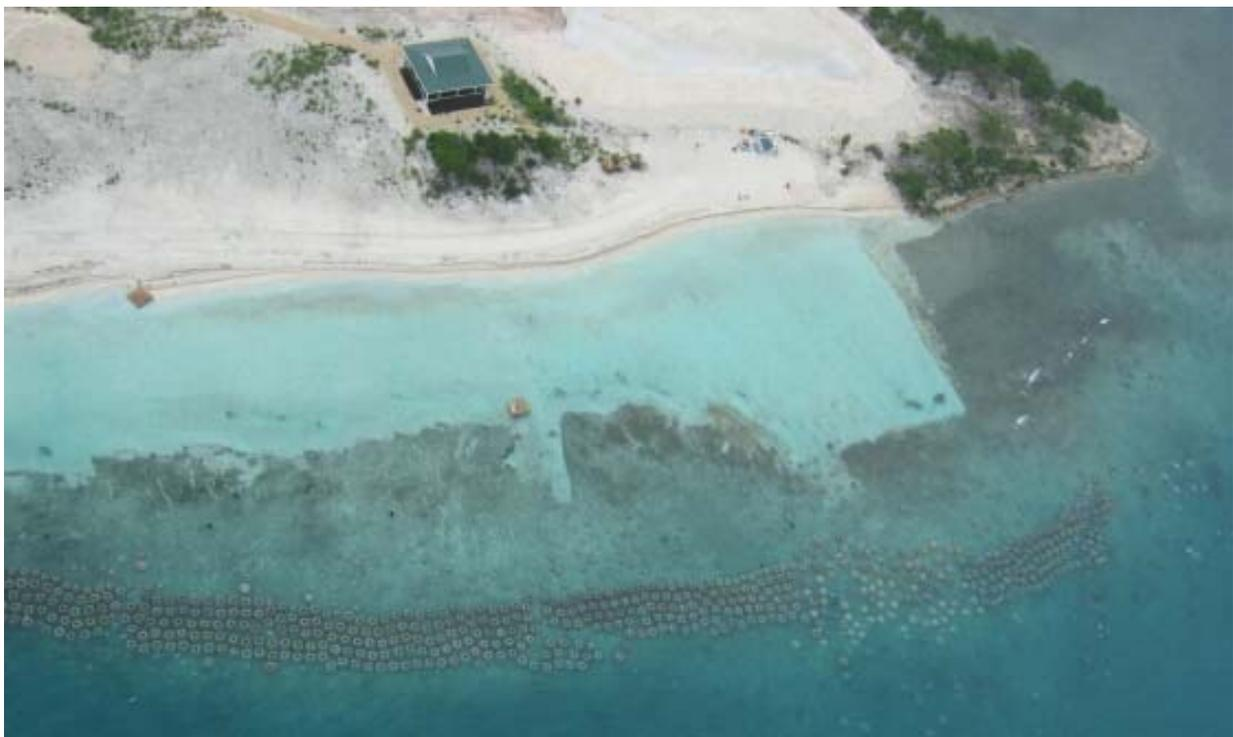
**Figure 8. Aerial Photograph of 5-Row Reef Ball Breakwater in Antigua**
