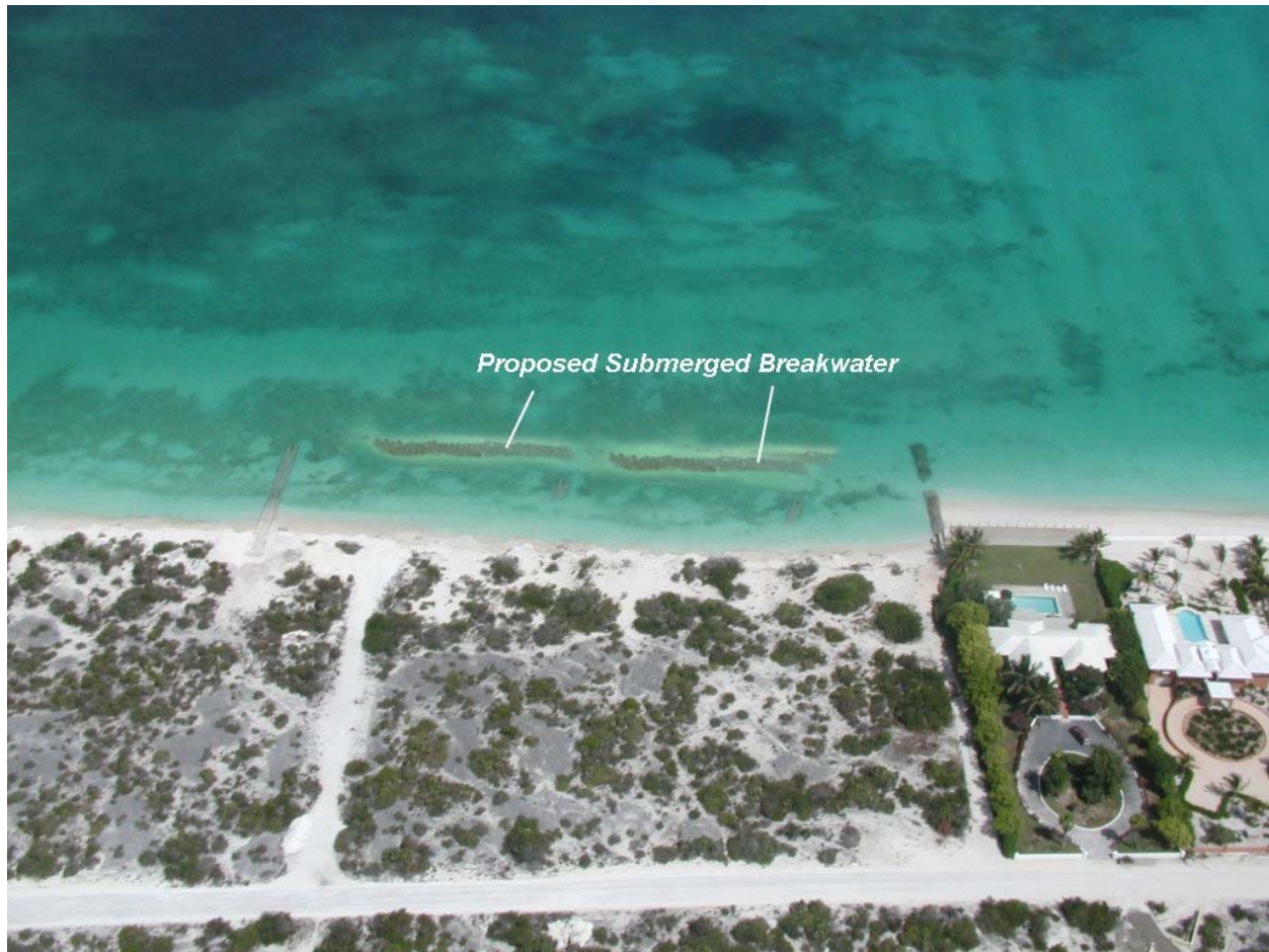
Figure 5. Conceptual Design of Offshore Submerged Artificial Reef Breakwaters
