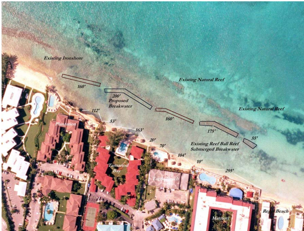
Figure 3. Proposed Reef Ball Breakwaters for Tamarind Bay & Adjoining Properties at South End of Seven Mile Beach (Dec. 2002 aerial courtesy DOE)
